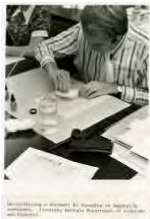
L-R: Deacidifying a document by sponging on magnesium carbonate (ca. 1975), sandwiching documents between layers of cellulose acetate and lamination film (1979), laminating sandwiched documents (1979). 4-1-57.
